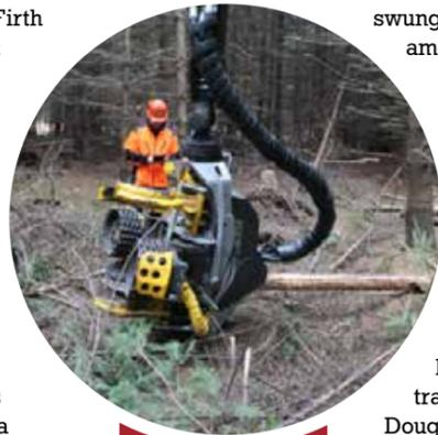
A visiting forester takes a close look at the Kesla 18RH2-II head. Upgrades to the tried-and-tested base machine now provide an ample power supply for the efficient operation of a crane and head normally suited to larger harvesters.
