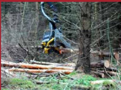
Top: Accurate positioning of the head for stem removal can be a difficult task in fast-grown young crops. The Kesla parallel crane geometry, responsive hydrostatic drive to the four wheels and the tilting system of the cab all assist in the speedy and precise positioning of the harvesting head.
