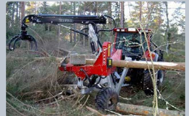
With its own load-sensing hydraulic system, it is operated with ECH mini joysticks from the comfort of the tractor cab. This machine comes with its own 7.5 m double extension crane and a 50 m radio-controlled winch to recover trees into range for the crane to then load onto the machine bed. It can also be fitted with the optional Hypro FG45 felling grapple to make it an all-round harvesting solution.
