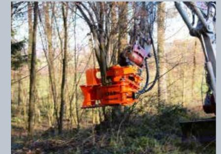
the chain coming off when cutting scrub as a patented design of guide bar is used on the saw unit. By using sequenced hydraulics no additional hydraulic or electrical connections are required when the Gierkink is being used on a crane. Gierkink have also patented their quick-attach system, which enables quick changing between the grapple saw and other attachments.
