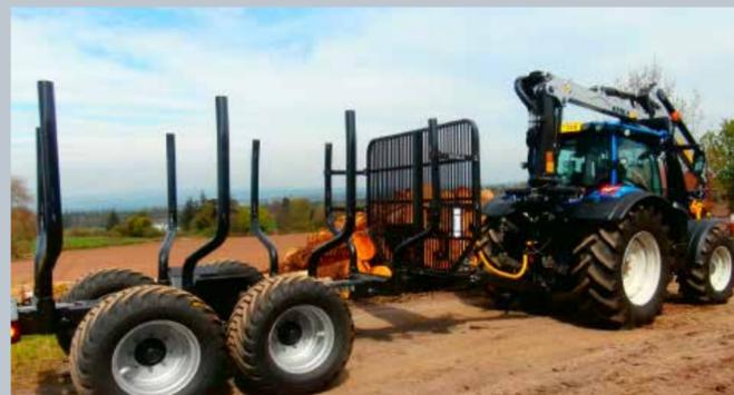
Latest in the range, the 7.5-tonne 720 model is designed for thinning and clearfell. With excellent manoeuvrability, the 720 is powered by a Cummins 97kw diesel engine and features reinforced NAF axles. A 180-degree swivel cab, air suspension and heated seat, air conditioning and CD radio are all standard. The simple coloured electronic display system enables easy machine operation and various parameters can be programmed for different drivers.
